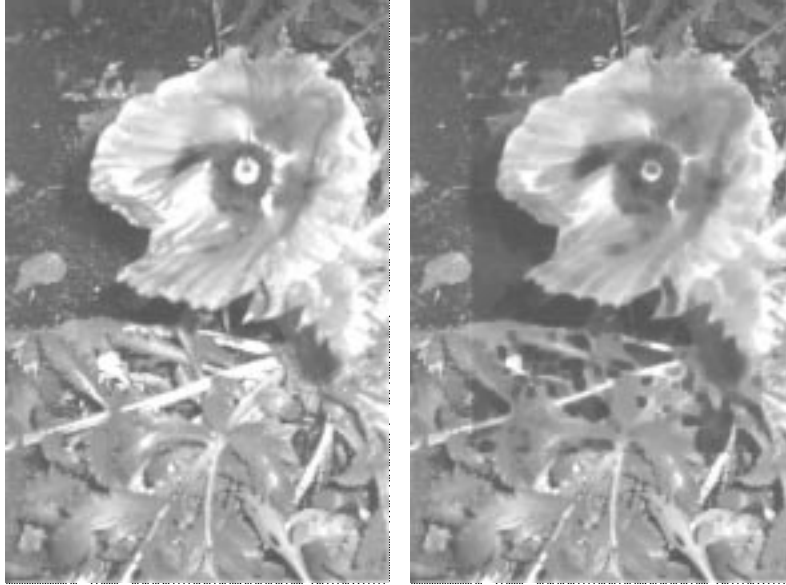
Figure 8-1 Erosion in a Rectangular ROI: the Source (left) and Result (right)
